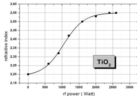
Figure 4: Refractive index variation of Titanium Oxides as a function of RF- Power.
