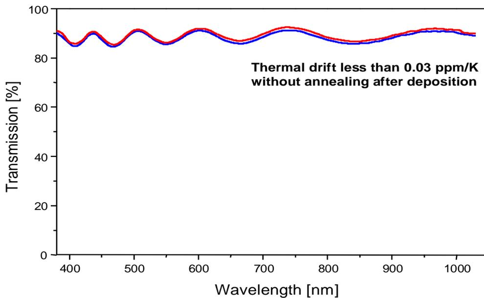
Figure 6: Spectral Data of a SiO<sub>2</sub> layer as deposited and after thermal annealing
