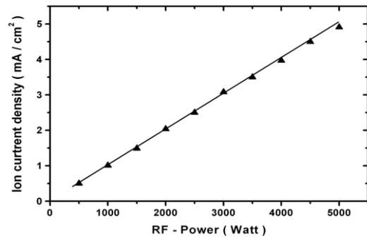
Figure 2b: COPRA ion current density variation as a function of RF-Power.
