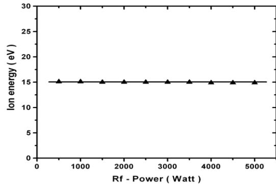
Figure 2a: COPRA ion energy variation as a function of RF-Power
