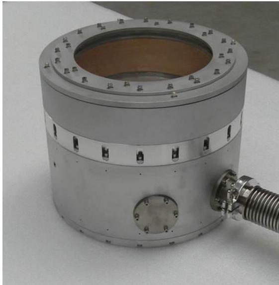
Figure 5: The COPRA IS300 in build source for controlled plasma beam assist during the deposition of precision optical coatings
